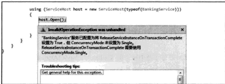
图 4-2 Multiple+ReleaseServiceInstanceOnTransactionComplete 导致的异常
