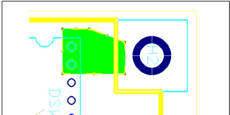
2. Select **Design»Shape to Area**. The copper is cut out to avoid the other elements within its area, as in the example shown below.
