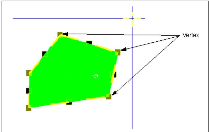
Complete the following steps to add a vertex to any line segment of a polygon:
