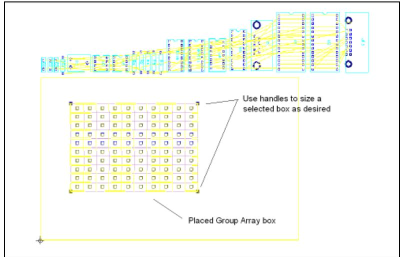
5. Begin selecting and dragging parts. As they are placed, the parts snap to the array.
