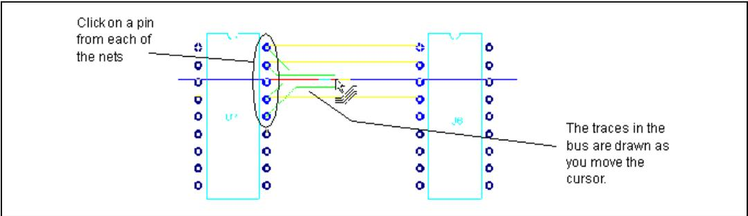
3. Move the cursor toward the bus's destination pins and double-click to complete copper placement.
