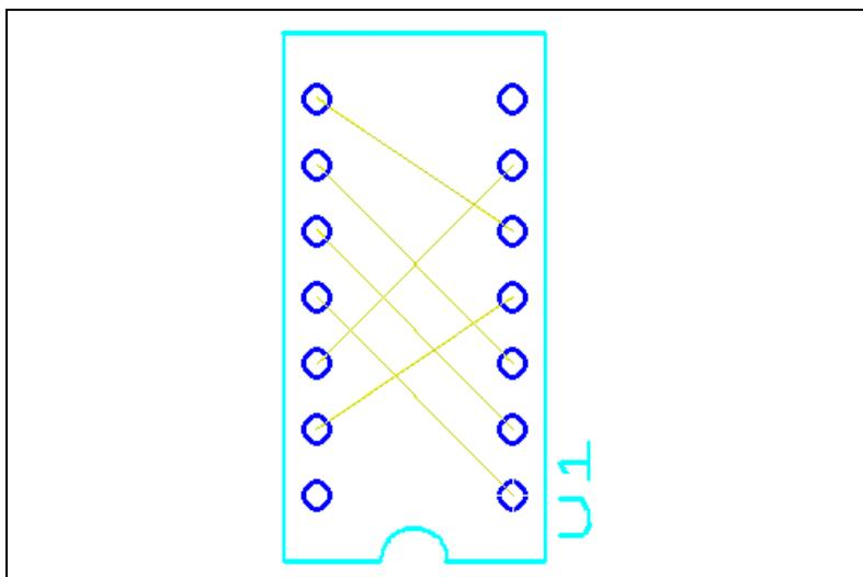
The above figure shows U1 before the automatic pin/gate swap. Note the position of the ratsnests.
