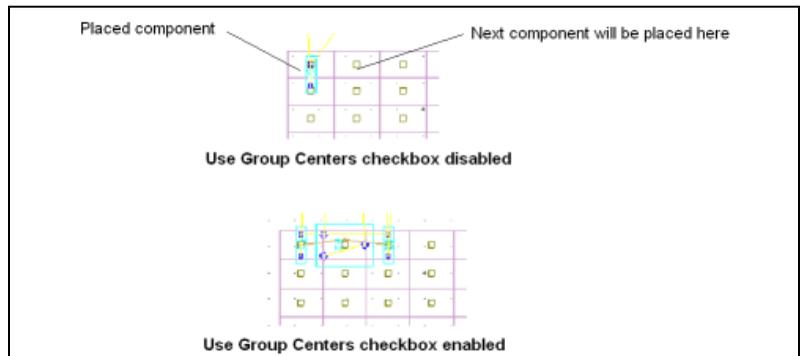
Place the part in the top left cell. The other parts will be placed at the same relative position in the other cells, beginning in the top left row and working to the right.
