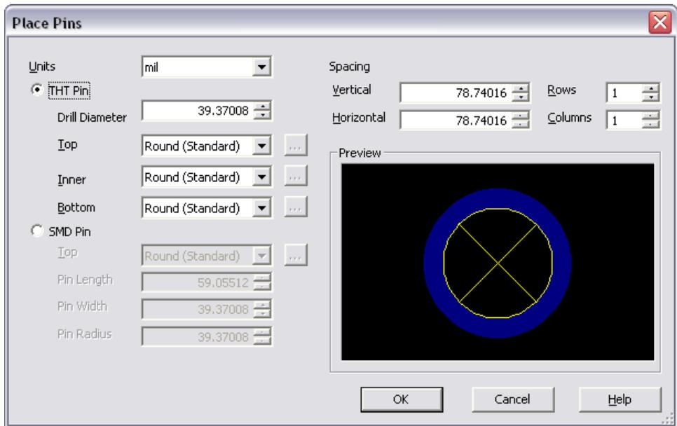
4. Indicate the pad type (THT or SMD) and its dimensions and spacing. Changes appear in the **Preview** panel. When you have made the necessary settings, click **OK**. The pin is attached to the pointer. Click on the part to place it.
