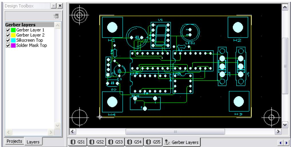
For Gerber RS-274X files, the layer name contained in the Gerber file is used as the layer name in the **Layers** tab. For example, “Silkscreen Top” and “Solder Mask Top,” as shown above.
