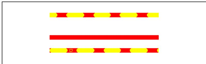
2. Select **Tools»Equi-space Traces**. The spacing between the traces is made equal, as shown in the example in the figure below.
