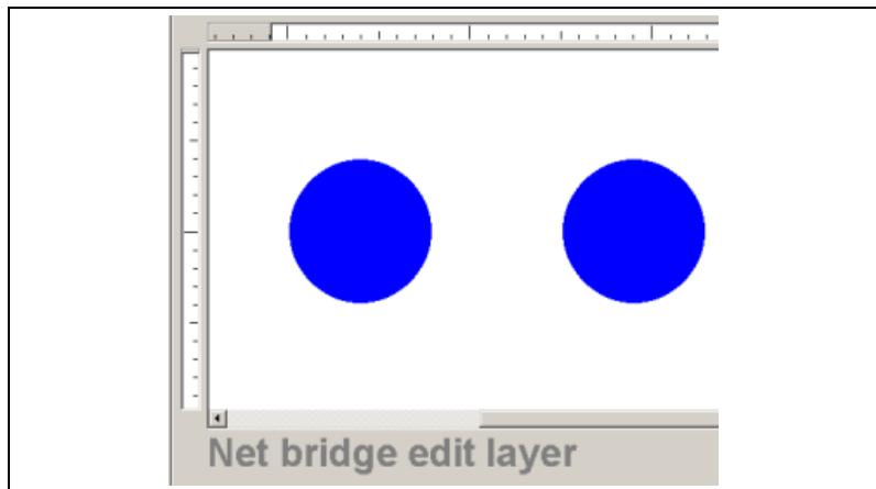
6. Connect the two pins by selecting **Place»Shape»Rectangle** and drawing a rectangle between them, being sure to overlap the two pins.
