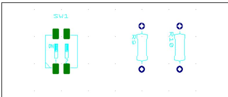
3. Click the **Add pins** button and click the desired pin in the workspace. Continue until all pins for the net are listed in the **Pins** area.
