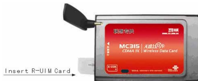
When MC315 card starts up, the lamp turns YELLOW. After a few seconds, the card will be ready to work, and the lamp turns GREEN.
