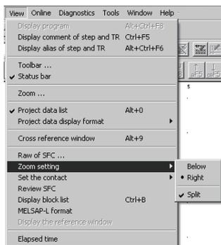
Choosing vertical partition or horizontal partition provides the corresponding one of the following displays.
