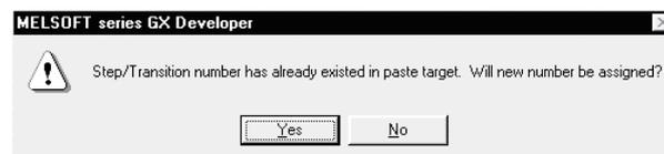
Choosing **Yes** executes pasting after the system has assigned a new number by reassigning lower to higher free numbers to the step/transition condition numbers of the pasting destination SFC diagram.
