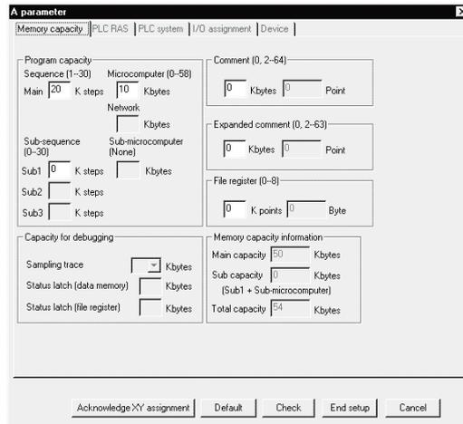
Set the microcomputer capacity and perform the operation of **Check** → **OK** → **End setup**.
