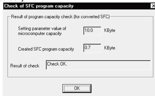
If "SFC program capacity is beyond the microcomputer cap." appears on the right of Result of check, PLC write or another format write cannot be performed as it will result in an error.
