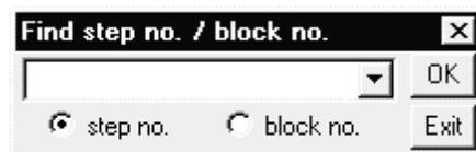
Clicking the **OK** button or pressing the **Enter** key allows the cursor to move to the specified step in the SFC diagram currently displayed.
