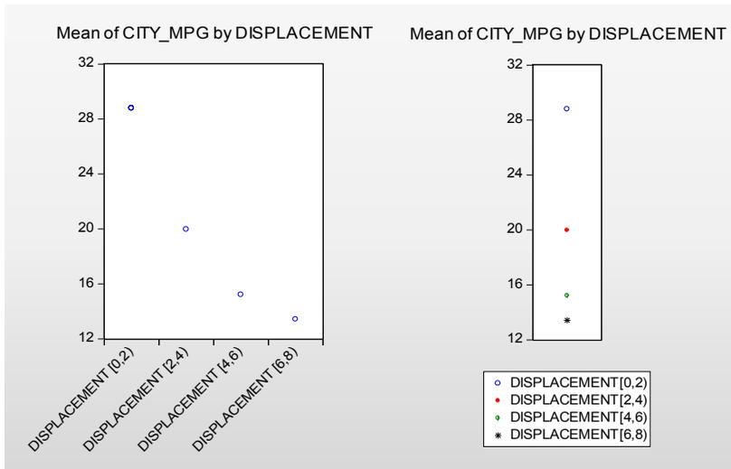
In the graph on the left, DISPLACEMENT is a primary factor so that each level of the factor is displayed as a separate “observation” along the axis using a common symbol and color for the dot. In the graph on the right, DISPLACEMENT is a secondary factor that is displayed
