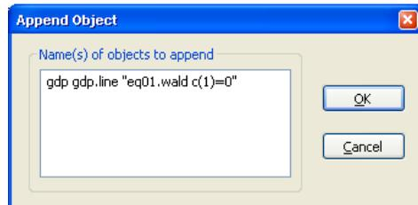
Note that when adding multiple outputs you should make certain to separate the names and commands by spaces. If necessary, you should enclose the text in double quotes, if, for example, the command statement includes spaces as in the Wald example above.
