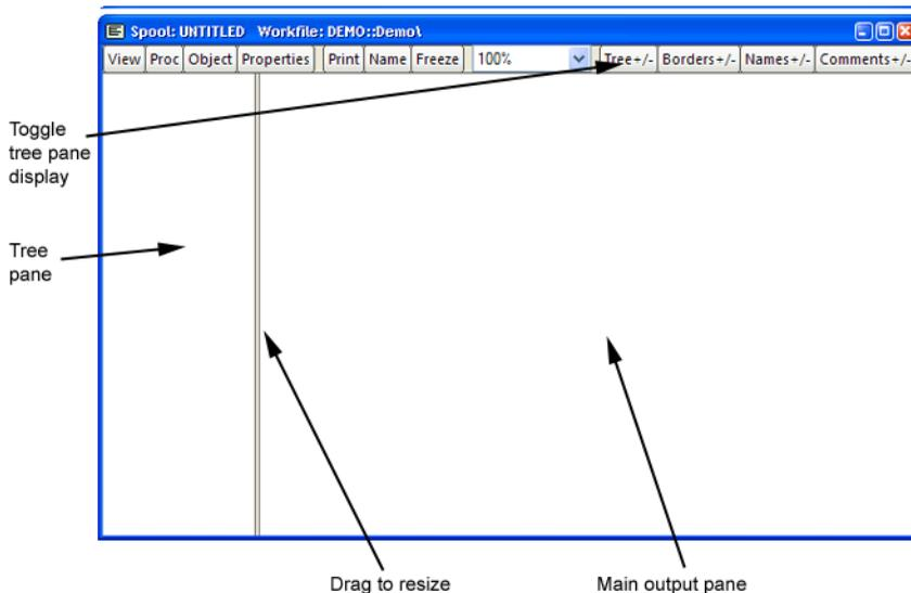
Here we see the spool view of an empty, unnamed spool object. As depicted here, the default is to display the contents of the spool using two panes. The left pane is the *tree pane*
