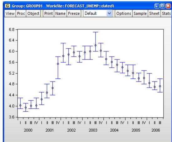
You may display an error bar graph for any group object containing two or more series; the error bar will use data for, at most, the first three series. To display an error bar graph, **View/Graph...** from the group menu, and then choose **Error Bar** in the **Specific** listbox.
