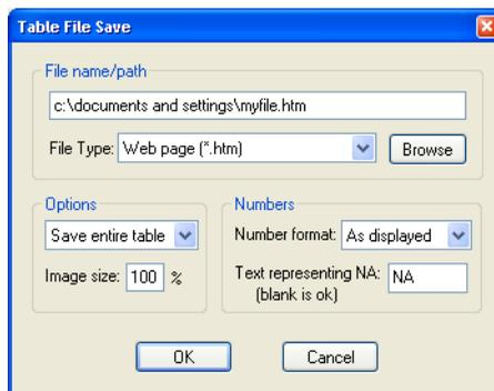
You may also specify options for how numbers are to be treated when written. You may specify a **Number format** so that numbers are written **As displayed** in the table, or using **Full precision**. In addition, you may change the text used to write missing values.
