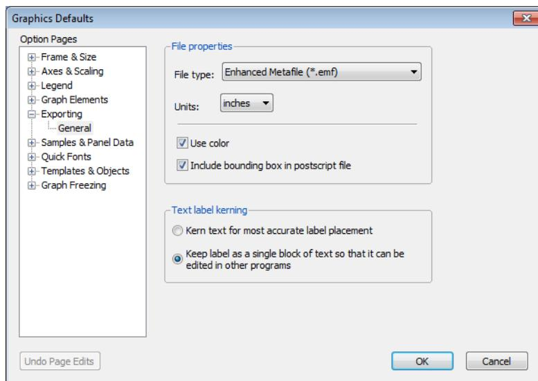
Additional dialog pages are provided for specifying the default settings for use when saving graphs to file (**Exporting**) and for handling sample breaks, missing values, and panel data structures (**Samples & Panel Data**).
