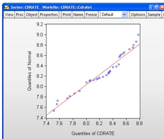
To display the theoretical quantile-quantile plot, select **View/Graph...** from the series or group menu, choose **Quantile - Quantile** in the **Specific** listbox, and select **Theoretical** in the **Q-Q graph** dropdown to the right.
