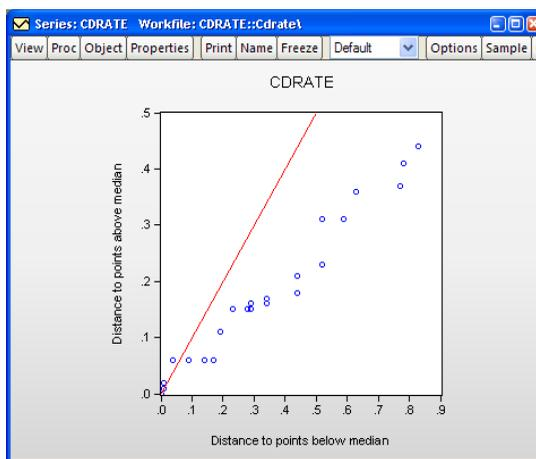
To display the quantile-quantile symmetry plot, select **View/Graph...** from the series or group menu, choose **Quantile - Quantile** in the **Specific** listbox, and select **Symmetry** in the **Q-Q graph** dropdown to the right.
