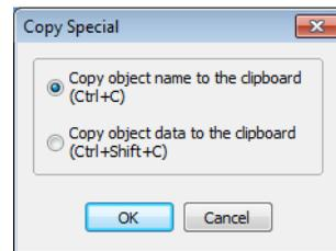
You can avoid the dialog by typing CTRL-C or CTRL-SHIFT-C, with the object selected in the workfile window.
