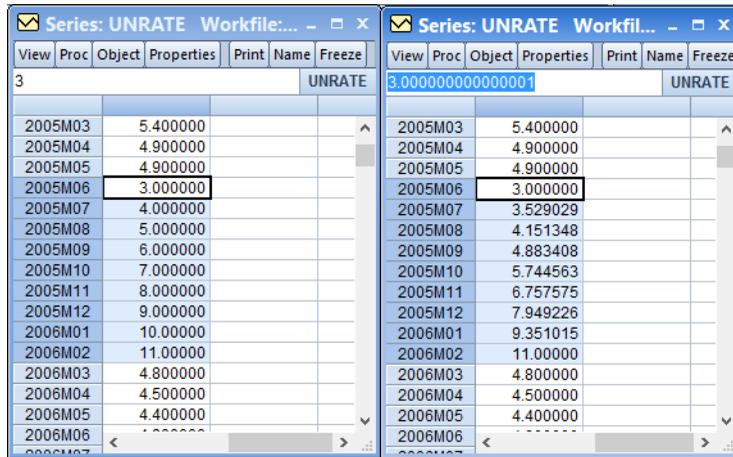
Since we have 9 cells selected, and we specified the values 3 and 11, linear interpolation (the left pane) is straightforward to calculate: the increase in each cell is constant, and equal to  $(11-3)/(9-1) = 1$ . The right hand pane shows multiplicative interpolation. Here, the increase in the log of each cell value is constant, and is equal to  $(\log(11)-\log(3))/(9-1)$ .
