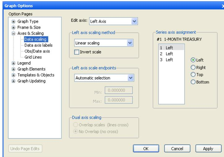
You may change the assigned axis by first highlighting the series and then clicking on one of the available axis buttons. For example, to plot several series with a common scale, you should assign all series to the same axis. To plot two series with a dual left-right scale, assign the two series to different axes. To edit characteristics of an axis, select the desired axis from the drop down menu at the top of the dialog.
