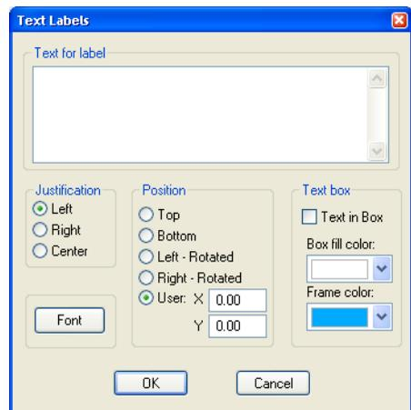
The first four options in **Position** place the text at the indicated (relative) position outside the graph. You can also place the text by specifying its coordinates. Coordinates are set in virtual inches, with the origin at the upper left-hand corner of the graph.
