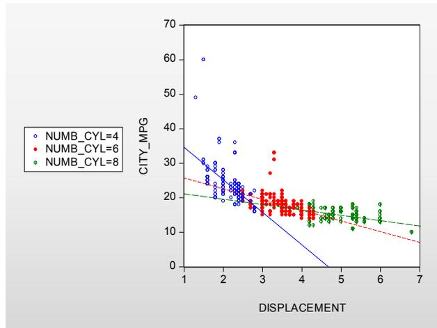
CITY\_MPG for cars as the number of cylinders increases, though the two high MPG outliers may be unduly influential in that comparison.
