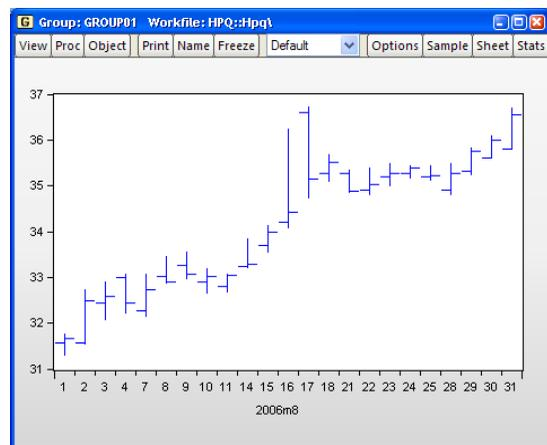
You may display a high-low graph for any group object containing two or more series. To display an high-low graph, **View/Graph...** from the group menu, and then choose **High-Low (Open-Close)** in the **Specific** listbox. Data for up to four series will be used in forming the graph.
