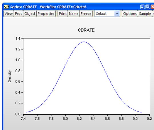
The **Options** button may be used to display the **Distribution Plot Customize** dialog. As with other distribution graphs, the left-hand side of the dialog may be used to add distribution graphs to the current plot (e.g., combining a histogram and a theoretical distribution).
