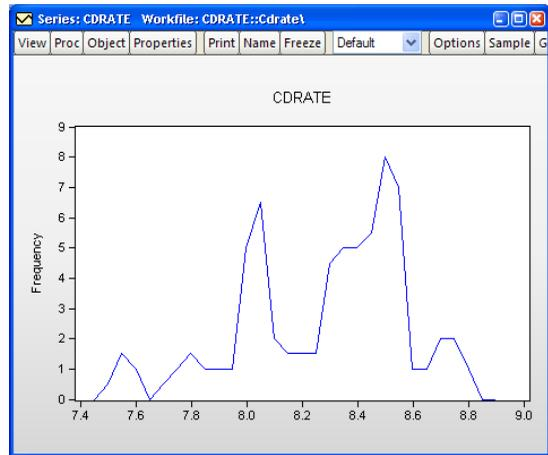
The default edge frequency graph for the CD rate data is displayed here. The EViews defaults, which were designed to generate easy to interpret histogram intervals, appear to undersmooth the data.
