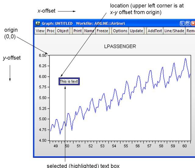
You can change the position of text added to the graph by selecting the text box and dragging it to the position you choose. After dragging to the desired position, you may double click on the text to bring up the **Text Labels** dialog to check the coordinates of that position or to make changes to the text. Note that if you specify the text position using coordinates, the *relative* position of the text may change when you change the graph frame size.
