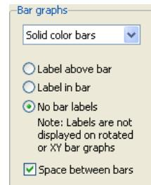
You may use the drop-down menu to apply fade effects to your bars. By default, EViews displays the **Solid color bars**, but you may instead choose to display **3D rounded bars**, **Fade: dark at zero**, **Fade: light at zero**. The latter two entries fade the bars from light to dark, with the fade finishing at the zero axis. Note that at press time, fades are not supported when exporting graphs to PostScript.
