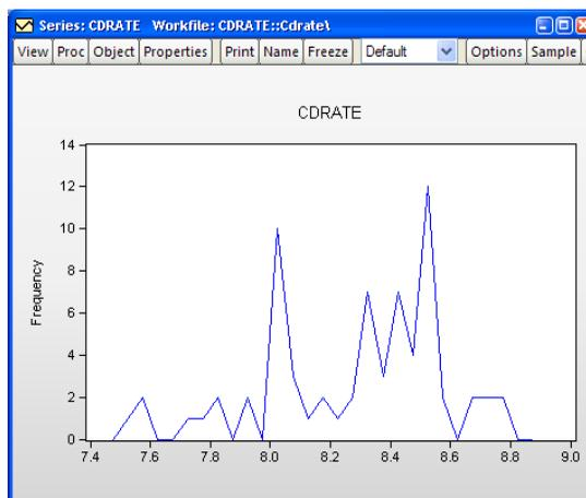
We use the default settings to display the frequency polygon for the three-month CD rate data. The EViews defaults, which were designed to generate easy to interpret histogram intervals, undersmooth the data.
