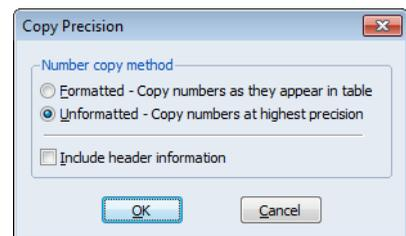
Additionally, if you are copying cells from a spreadsheet, you may choose to **Include header information**. This will also copy the column and row labels for the selected range of cells.
