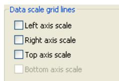
Notice that the **Bottom axis scale** checkbox is disabled in the image to the right. This indicates that the date scale for our current graph is assigned to the bottom axis, so the **Obs & Date axis grid lines** group should be used to control grid lines for this axis.
