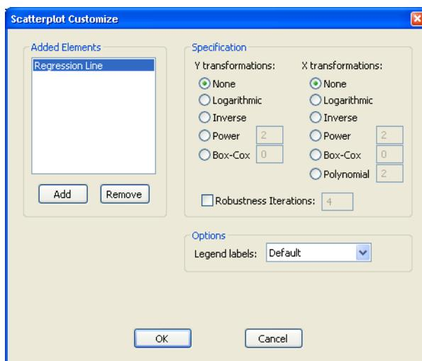
First, you may specify transformations of your dependent and independent variables using the radio buttons. The following transformations are available for the bivariate fit:
