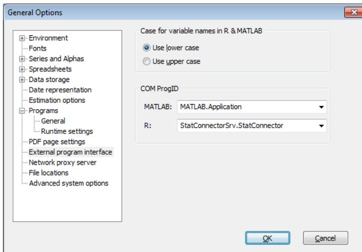
You may also use the **COM ProgID** section of the dialog to specify the default Programmatic IDs (ProgIDs) used when instantiating a MATLAB or R COM server. The ProgID is used to indicate the version of MATLAB or `statconnDCOM` to which EViews connects when you
