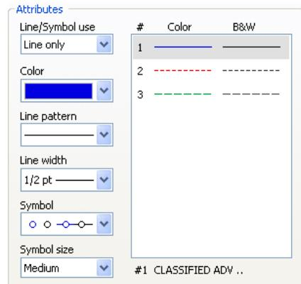
The **Line/Symbol** use dropdown determines the combination of lines and symbols used to display the selected element. You should change the **Line/Symbol** use dropdown to **Line & Symbol** to display both lines and symbols, or **Symbol only** to suppress the lines. The corresponding **Color**, **Line pattern**, **Line width**, **Symbol**, and **Symbol size** dropdowns control the characteristics of the selected element. Note that the settings will sometimes have no
