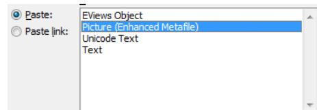
A metafile will be inserted into your Excel document. The static image can only be resized and edited using the tools within Excel. It is not connected to EViews in any way.
