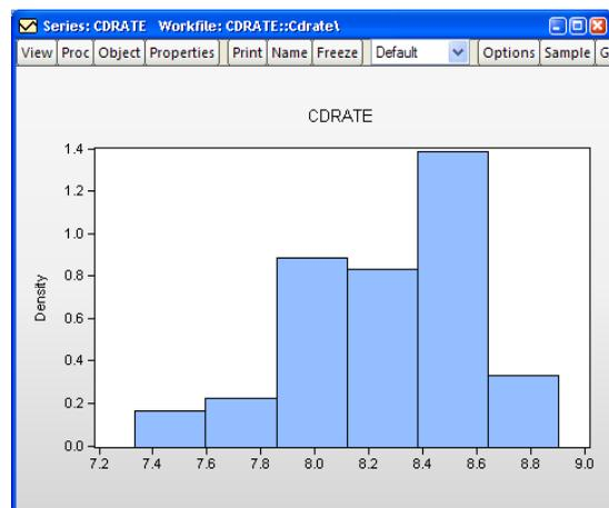
The **Right-closed bin intervals** checkbox controls how observations that equal a bin endpoint are handled. If you select this option, observations equal to the right-endpoint of a bin
