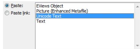
(Note that this static **Paste As Text** mimics the default Excel paste operation. You can perform this operation by selecting the **Paste** button or pressing CTRL-V. However, you should use **Paste Special...** to specify a paste of **Unicode Text**.)
