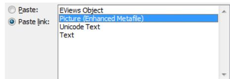
from the listbox and click **OK**. If the link option is grayed out in the dialog, remember that the EViews workfile and the object you copied from must be named before pasting as a link.
