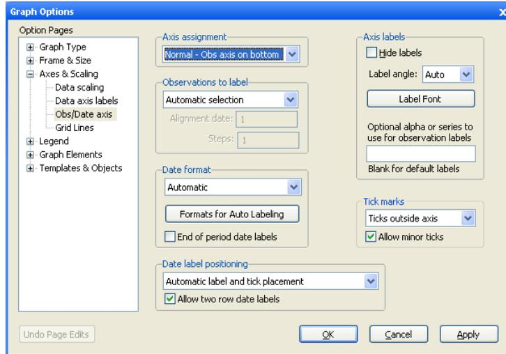
For graphs which do not have a date axis, such as XY graphs, the **Axis assignment** drop-down menu in the top left-hand corner of the page will read **Graph has no Obs/Date axis**, and any changes to the settings on this page will be irrelevant for the current graph type.
