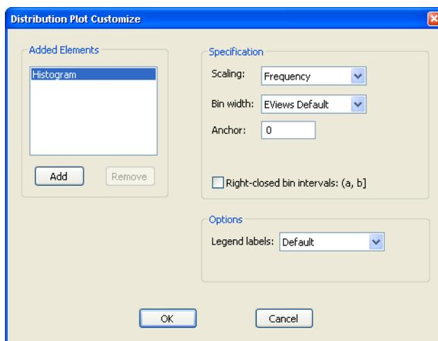
First, the **Scaling** dropdown menu lets you choose between showing the count of the number of observations in a bin (**Frequency**), an estimate of the density in the bin (**Density**), and the fraction of observations in each bin (**Relative frequency**). The density estimates are computed by scaling the relative frequency by the bin width so that the area in the bin is equal to the fraction of observations.
