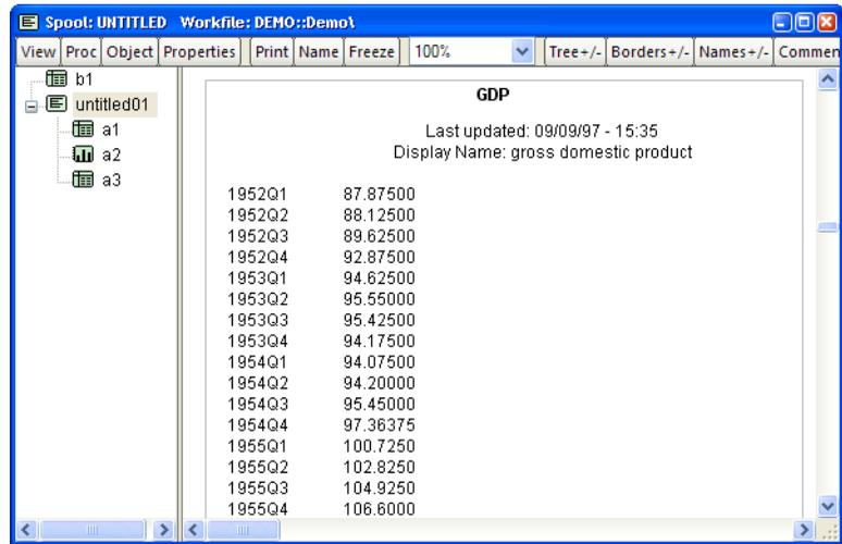
with the three output objects in the embedded spool displayed in the branch of the tree. Clicking on B1 in the root of the tree scrolls the output window so that B1 is displayed in the main output pane; clicking on A1 in the UNTITLED01 branch of the tree scrolls to the A1 output object from MYSPOOL. As with all tree structures, you may click on the tree icon next to UNTITLED01 to open or collapse the display of the branch.
