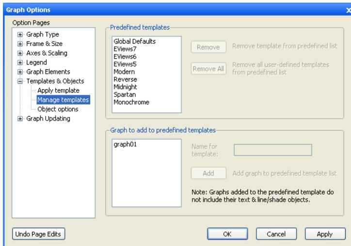
To add a graph to the predefined template list, select it from the listbox on the bottom and click the **Add** button. The graph will then move into the predefined list on the top of the dialog and will be removed from the list on the bottom. Before clicking the **Add** button, you
