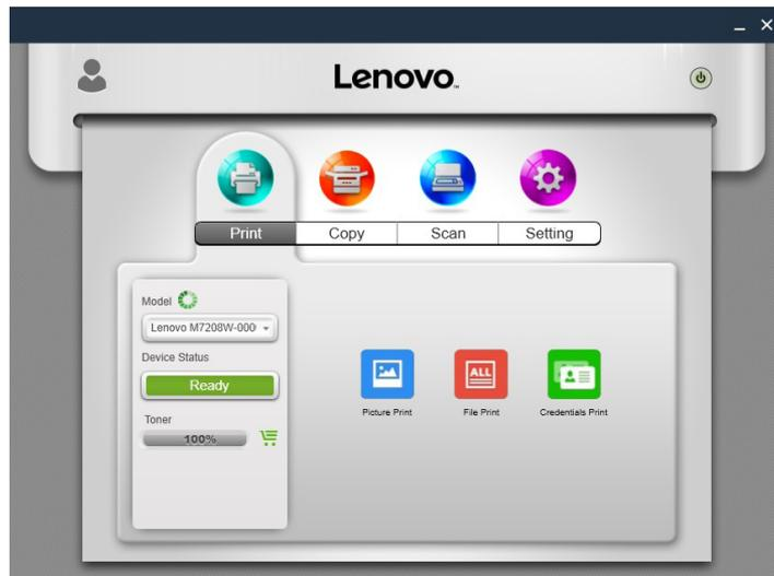
The Toner option shows the level of toner remaining in the printer. When the toner level falls to 30%, 20%, 10%, or 5% the shopping cart icon will flash as a reminder.
