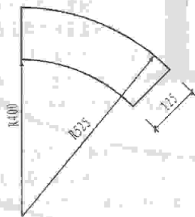
C30预制混凝土砌块大样
