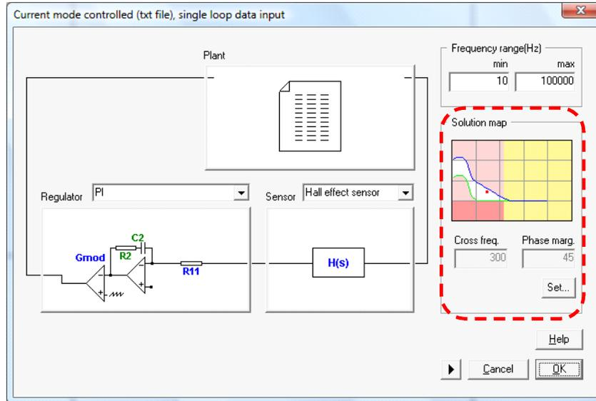
Now accept the selected configuration and confirm the design, the program will automatically show the performance of the system in terms of frequency response, etc.
