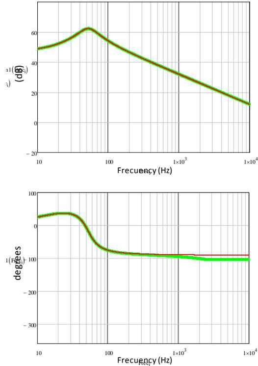
Once the frequency response is obtained, in PSIM, go to **Utilities** -> **Launch/Export to SmartCtrl** (or click on the icon **Run and Export to SmartCtrl**) to export the ac sweep result to SmartCtrl.
