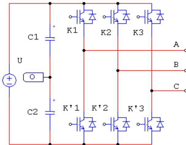
We can create a three-phase voltage source inverter by grouping together three single-phase half bridges and a capacitor voltage divider.
