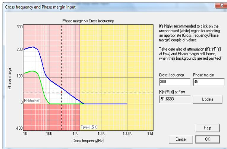
Once the crossover frequency and the phase margin have been selected, the solution map will be shown on the right side of the input data window. If, at any time, these two design parameters need to be changed, just click on the shown solution map (See next figure).
