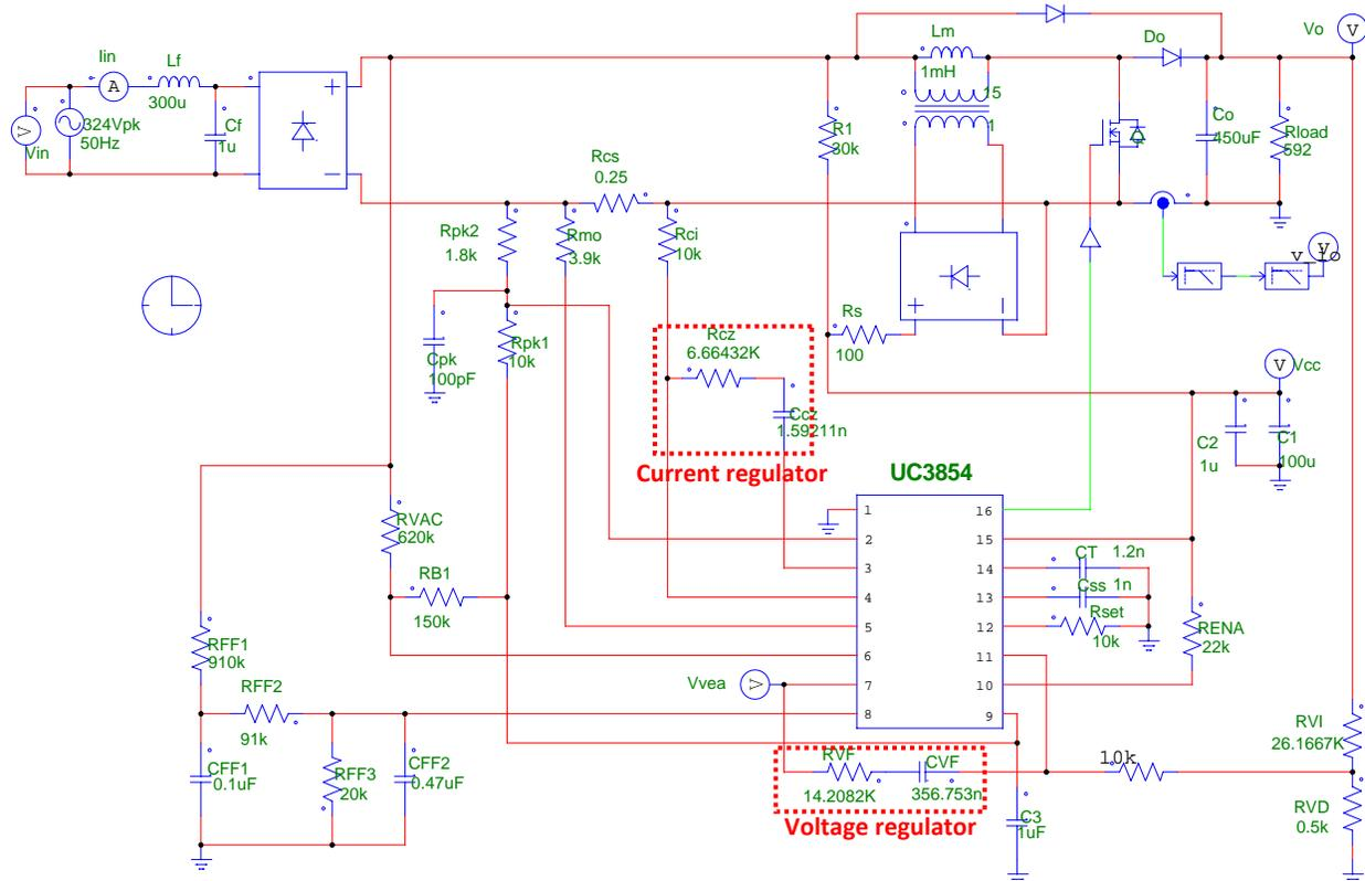
The circuit includes the inner current loop and the outer voltage loop. The current loop regulator parameters are the resistance  $R_{cz}$  and the capacitance  $C_{cz}$ , and the voltage regulator parameters are the resistance  $R_{vf}$  and the capacitance  $C_{vf}$ , highlighted in the red dotted boxes above.
