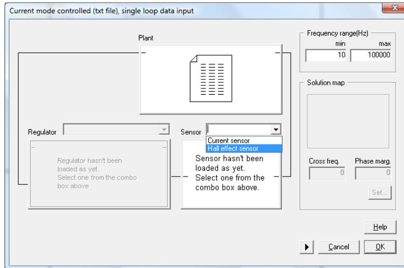
In this case, the hall effect sensor is selected. Then define the sensor gain and the bandwidth (pole frequency) of the Hall effect sensor.
