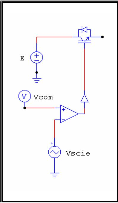
It is possible to improve the model by taking into account the delay induced by the chopper. In dynamic state the voltage  $V_{com}$  varies in time so that the response of the chopper is not instantaneous.
