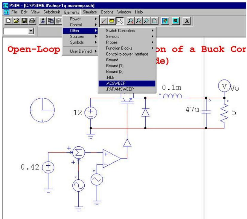
Place the AC Sweep block on the circuit :
