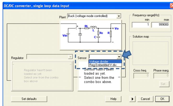
In the case of a voltage divider, one must enter the reference voltage. SmartCtrl will automatically calculate the sensor gain. In this example, the reference voltage is set at 2.5V. The figure below shows the sensor input data window.
