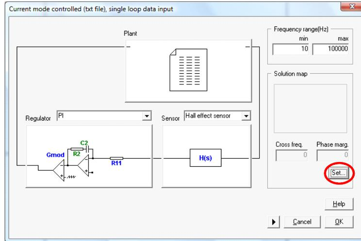
Now, select the crossover frequency and the phase margin of the loop just by clicking within the white zone and click OK to continue. The selected pair (PM and  $f_{cross}$ ) will provided stable operation. Optimization process could be carried out in the main SmartCtrl window.
