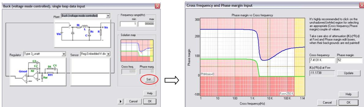
The x-axis of the Solution Map represents the crossover frequency, and the y-axis represents the phase margin. A design point in the Solution Map, therefore, defines the crossover frequency and the phase margin of the control loop. The white region of the Solution Map indicates the area where the design point should be placed. Click in the white region to define the crossover frequency and the phase margin. Then click on **OK** to exit the Solution Map dialog window.
