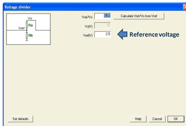
Note that the design will be carried out using this gain, and the resistor values to implement the voltage divider will be listed by SmartCtrl together with the regulator component values.
