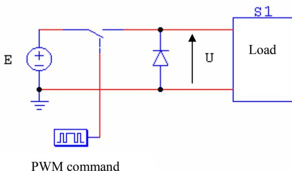
In general a chopper feeds an inductive load. This is the case of a load from a DC motor. The free-wheel diode prevents voltage surges due to commutation of an inductive load and protects the controlled switches. This one quadrant chopper is not reversible.
