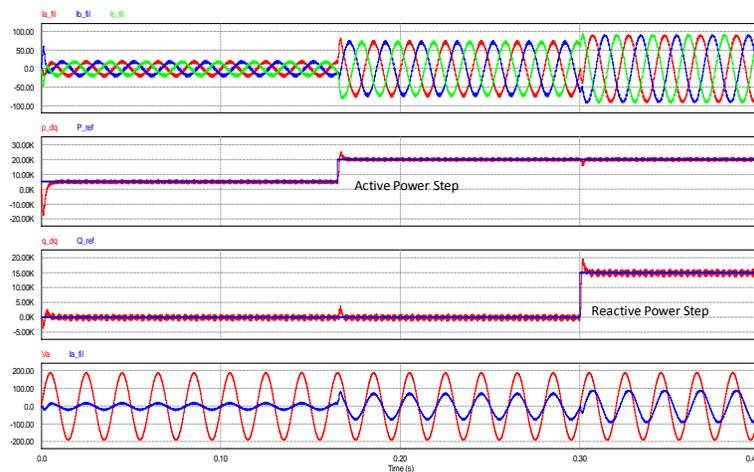
As it can be seen from the simulation results, the control loop, designed in SmartCtrl and validated in PSIM, provides a good performance to the 3-phase PV inverter system without the use of feedforward decoupling loops.
