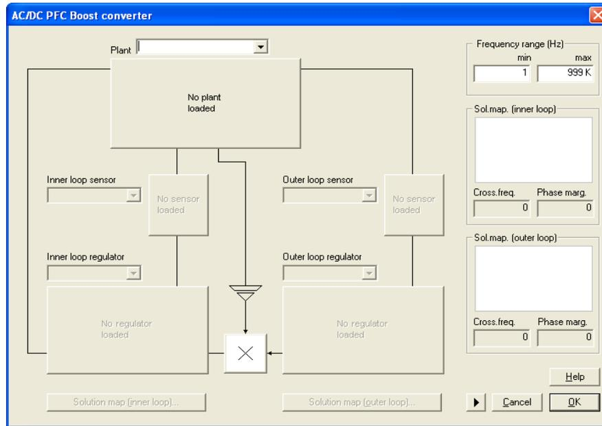
The PFC boost converter is controlled by a double loop control scheme. The inner loop is a current loop, and the outer loop is a voltage loop. Note that the PFC boost converter design must be carried out sequentially. The SmartCtrl program will guide you through this process.
