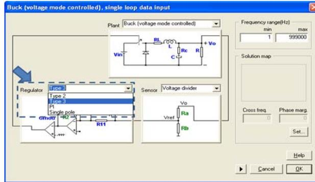
The type of regulator depends on the plant controlled. In this example, since the plant is a second order system, the best choice is a Type 3 regulator in order to obtain the proper phase margin and enough bandwidth. Select the Type 3 regulator, and enter the parameters as shown below, where  $G_{mod}$  is the modulator gain.
