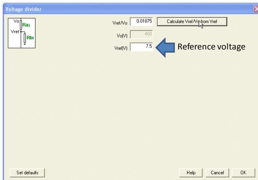
Then press on “Calculate Vref/Vo from Vref” button to set the attenuation of the voltage divider.
