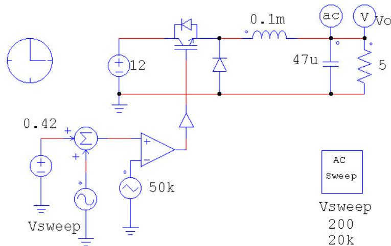
The principle of the AC analysis is that a small AC excitation signal is injected into the system as perturbation and the signal, at the same frequency, is extracted at the output.
