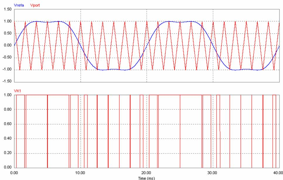
In this case the equation of the reference voltage is written:  $V_{ref} = r \sin \omega t + k \sin 3 \omega t$
