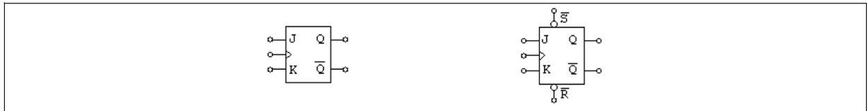
A J-K flip-flop is positive edge triggered, and the truth table is:
