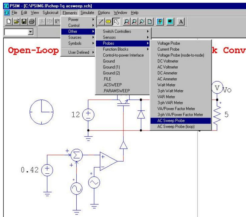
Place the AC Sweep Probe (ACSWEEP\_OUT) at the desired output location :
