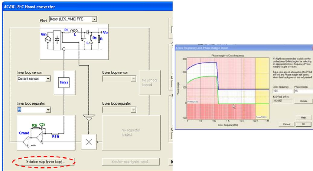
Once the crossover frequency and the phase margin are selected, the Solution Map will be shown on the right side of the converter input window. If, at any time, one needs to change the crossover frequency or the phase margin, click on the white area of the Solution Map, as shown in the figure below.
