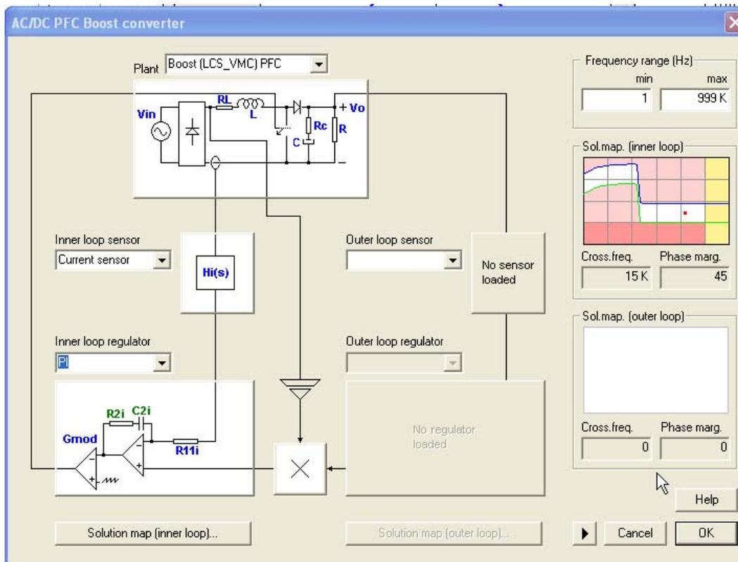
Once the inner loop design is completed, one can move on to the outer loop design.
