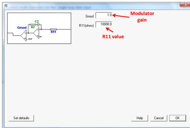
For an equivalent analog implementation of the compensator, it is necessary to set the modulator gain and the value of the resistance “R11”. In this case the resistance value is not important because the PI regulator to be implemented in PSIM is given by the values of the proportional gain and the time constant in s-domain transfer function block diagram.
