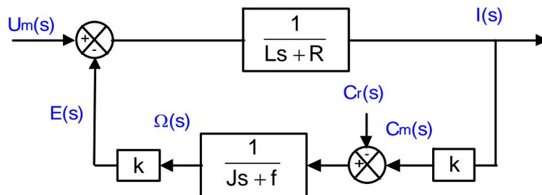
This block diagram will be used to study current control (or torque control). It will also be useful to set the parameters of the current circuit in the case of speed control with a secondary loop.
