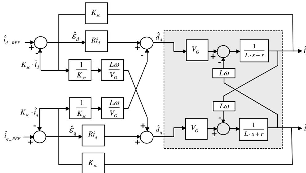
Due to the axis decoupling, this approach requires large amount of computations. For low cost applications (low cost  $\mu$ P, PIC, DSP or small FPGA), a simplified control strategy is needed, as shown in the next figure. In the simplified approach, direct PI control (without feedforward paths for axis decoupling) is used.
