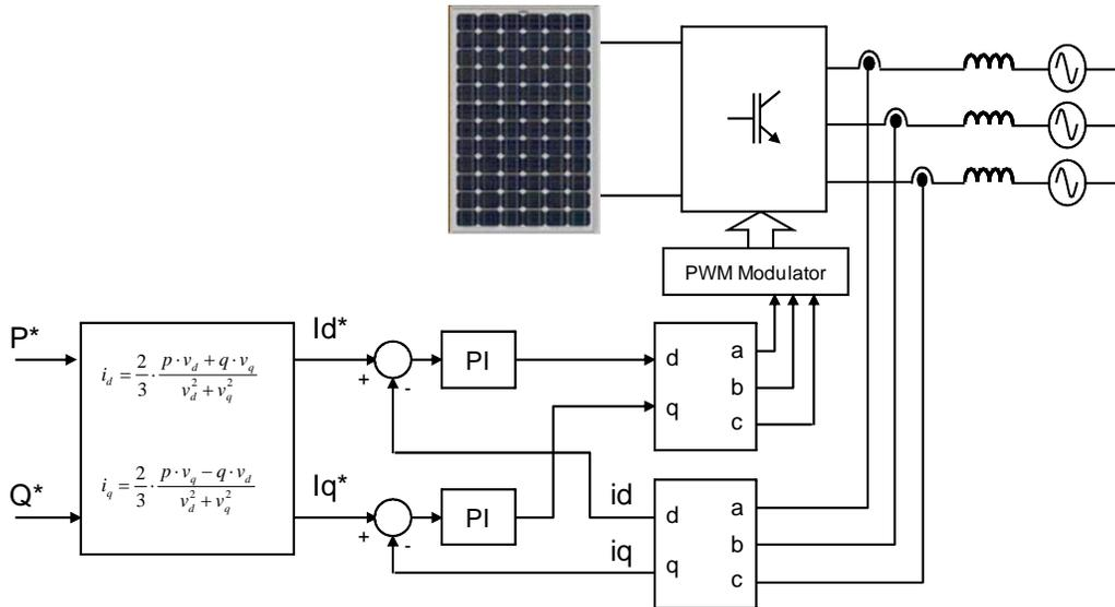
There are different ways to control such a system. One approach is to use the axis decoupling by means of feedforward control as shown in the figure below.
