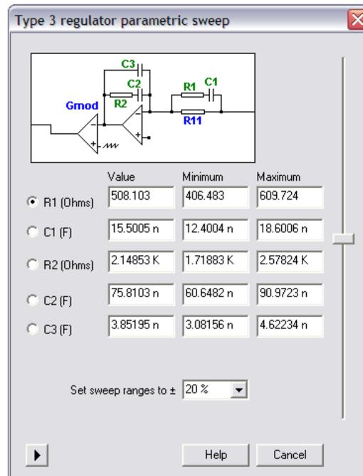
After selecting a particular parameter, one can change the slide bar and see instantly how the change of this parameter affects the control loop performance.
