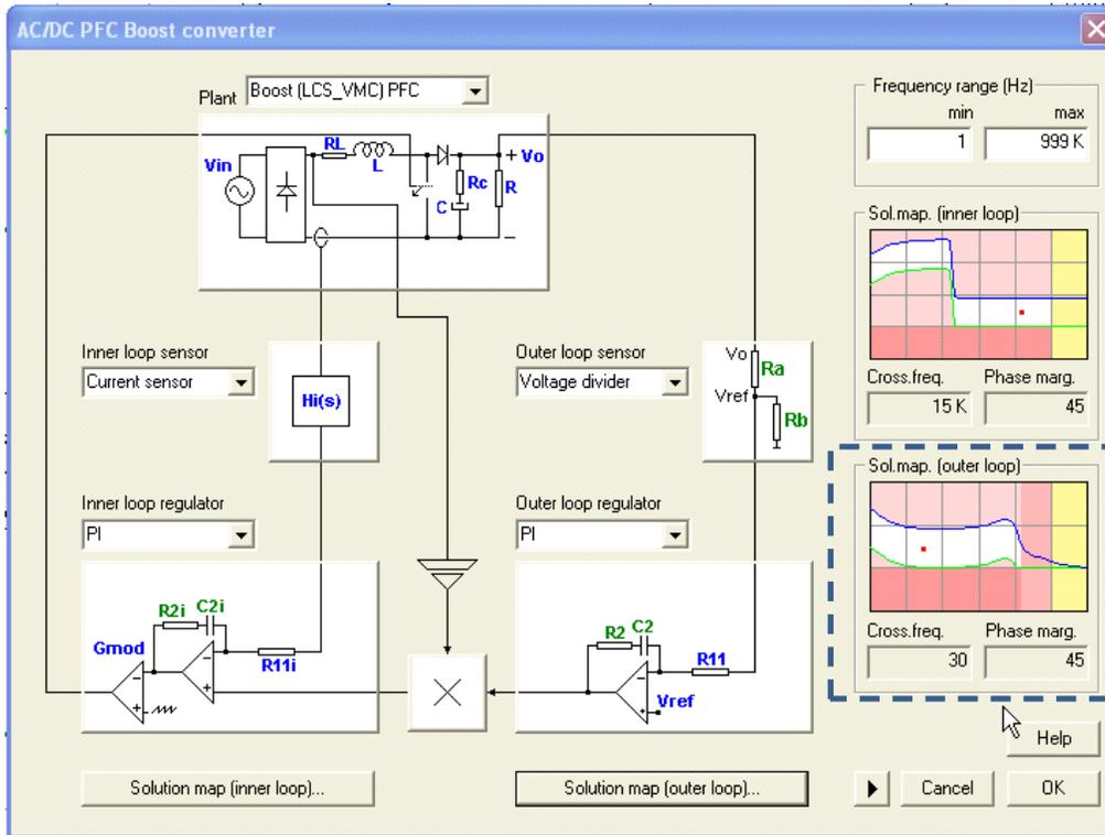
Accept the selected design by clicking on OK. The program will automatically show the control system performance by means of the Bode plots, the Nyquist plot, phase margin, etc.
