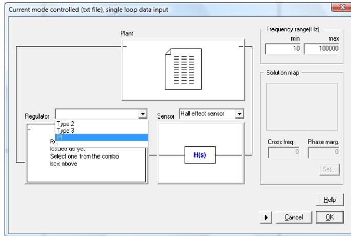
The PI regulator is selected in this case. The PI regulator specification window is shown below.
