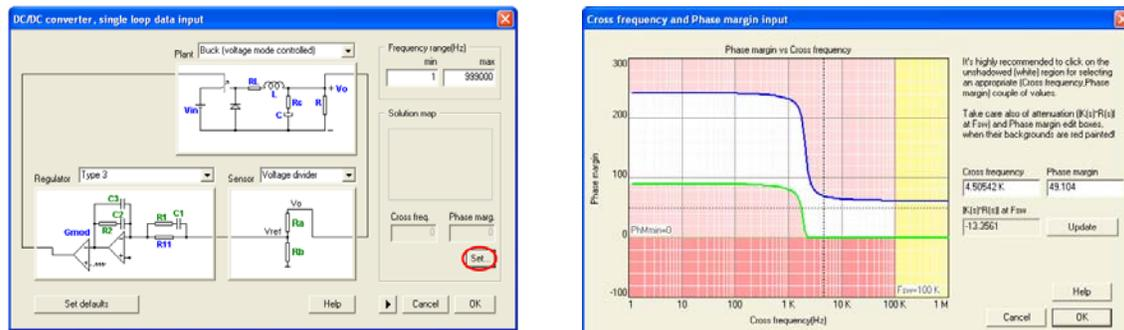
The x-axis of the Solution Map is the crossover frequency and the y-axis is the phase margin. Based on the converter parameters and the type of regulator selected, SmartCtrl will generate a safe
