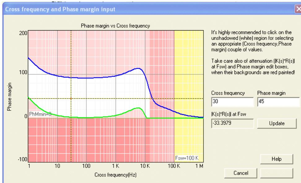
Once the crossover frequency and the phase margin are selected, the Solution Map will appear on the right side of the converter input window. If, at any time, these two parameters need to be changed, click in the white area of the Solution Map, as shown in the figure below.
