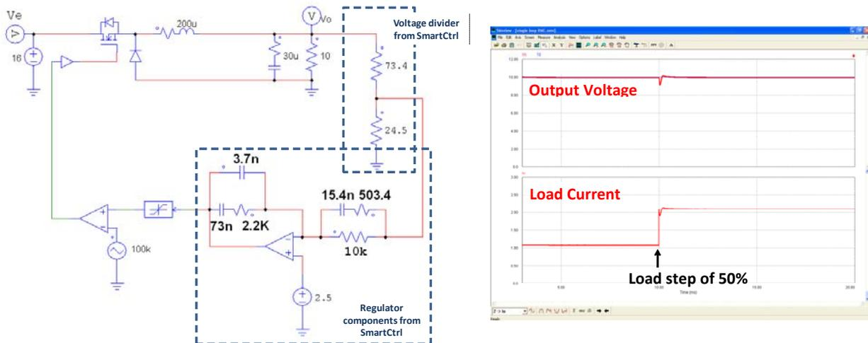
The example illustrates that SmartCtrl in combination with PSIM provide a fast and powerful platform for the design and validation of power converter control.
