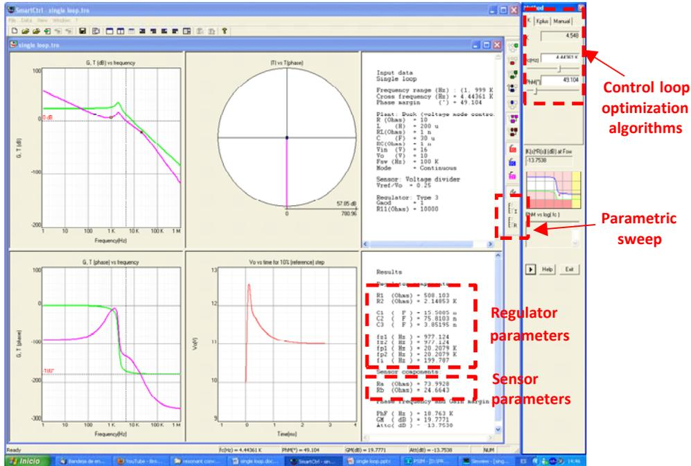
Additionally, by selecting **Data -> Parameter sweep -> Input parameters** or **Regulator components** in SmartCtrl, one can perform sensitivity analysis. The figure below shows the dialog windows of the parameter sweep for input parameters and regulator parameters.
