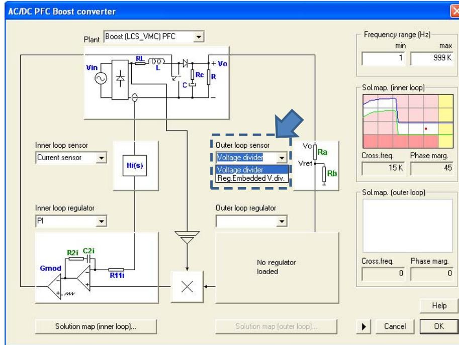
When using a voltage divider, one must enter the reference voltage, and the program will automatically calculate the sensor gain. In this example, the reference voltage is 7.5V. The sensor input data window is shown below.
