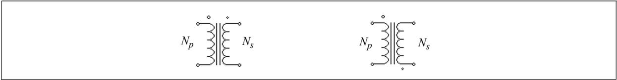
The winding with the larger dot is the primary, and the other winding is the secondary.
