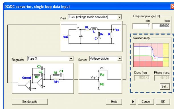
Now click OK to confirm the design, and the program will automatically show the performance of the system in terms of the Bode plots , polar plot, transient response, etc.
